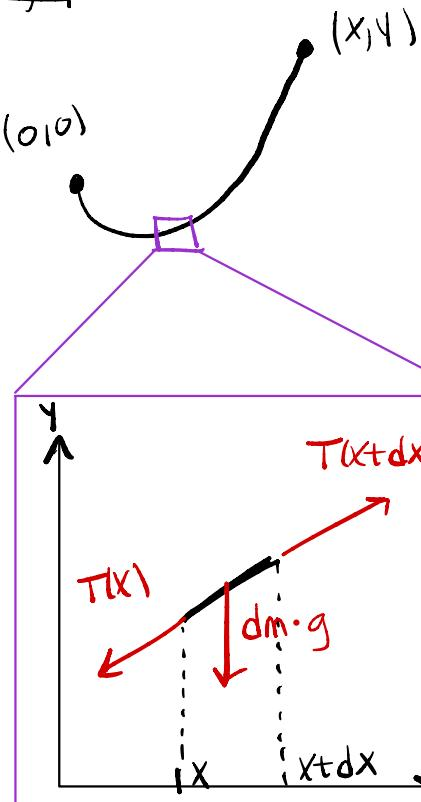
What is the shape of a rope of mass  $m$  and length  $l$ ?
